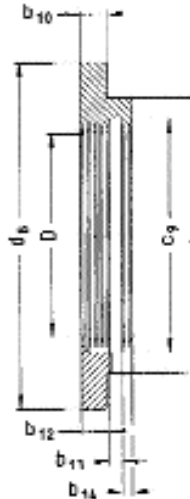
Type 20 rigid seal with two insulated labyrinth systems dimension b_{10} + 3 mm protection grade IP 44
